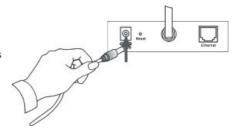
TIP: You can confirm power source is supplied from the LED indicators label Power on the Pan/Tilt Internet Camera is illuminated.
